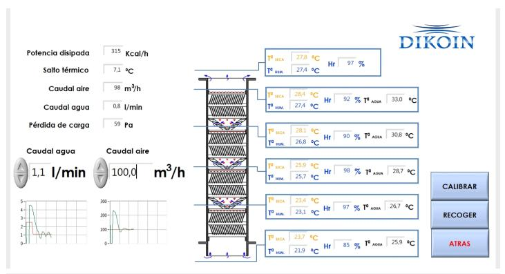
The equipment includes a PC with software to manage the equipment. In it, all the control points of the equipment are shown, and the data adquisition is permited in manual or automatic mode.
