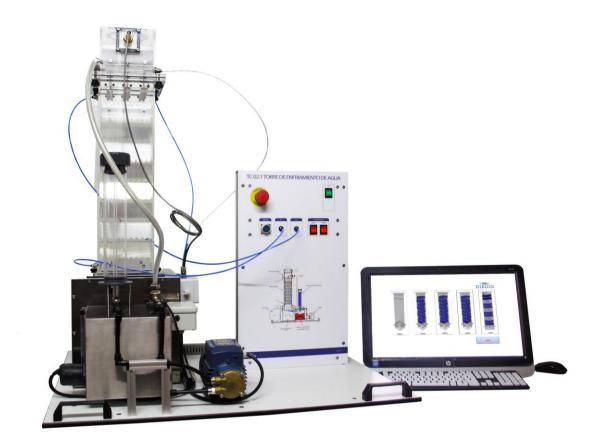
The TC 02.1 unit operates a standard cooling method, used in the industrial sector. This method involves cooling hot water to environment temperature.
